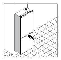
Open the door and push the appliance against the side of the kitchen unit opposite to that of appliance hinges.
